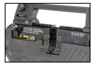
In order to install the magazine, the rifle will first need to be cocked. Pull the cocking handle all the way to the rear and lift it up into the cocked position.
