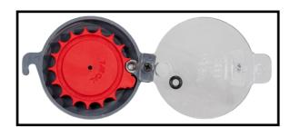
3) Load one pellet into the magazine, inline with the opening of the magazine body. This pellet will hold the magazine in the wound position.
